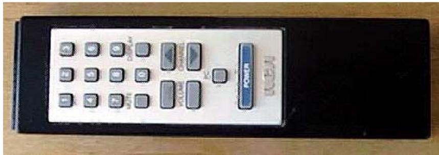
The remote control's job is to wait for you to press a key, and then to translate that key-press into infrared (pronounced "infra-red") light signals that are received by the TV. When you take off the back cover of the control you can see that there is really just 1 part visible: a printed circuit board that contains the electronics and the battery contacts.
