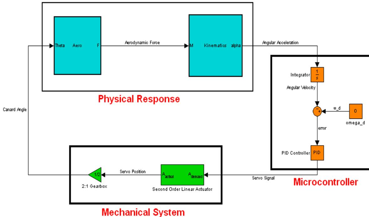
Figure 2. Overall schematic of the guidance control system where it data from the physical response will be process in the microcontroller before sending to the servo to control the rocket.
