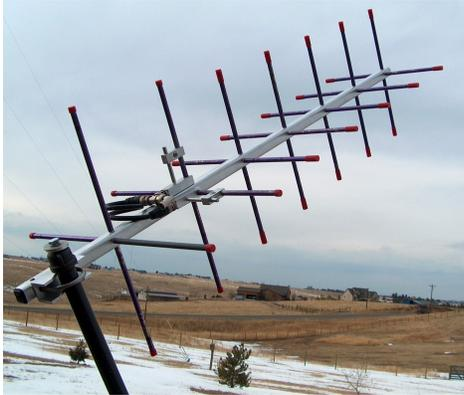
Figure 6– Circular polarized Yagi antenna
