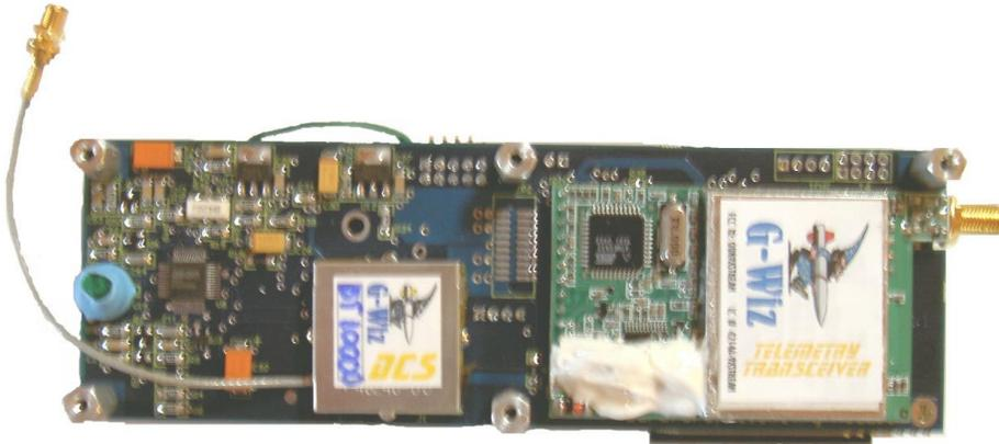
Figure 4 – G-Wiz DCS Flight Computer bottom view
