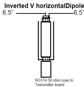
Figure 7 – Inverted V-horizontal dipole antenna
