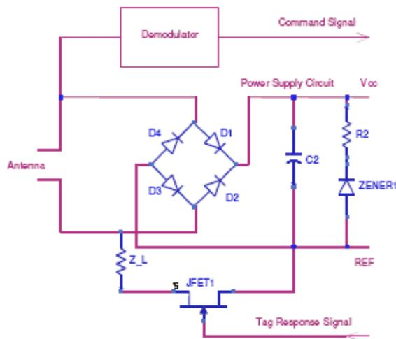
Figure 3: Powering an RFID Chip
