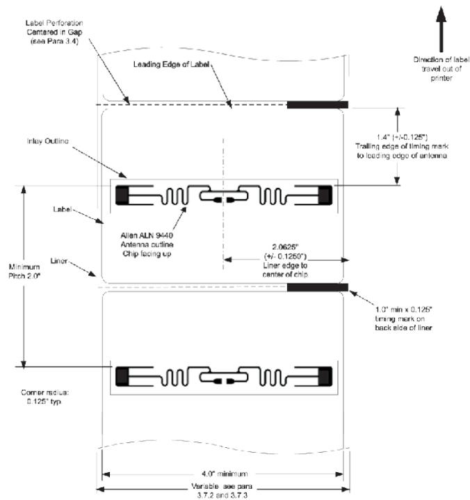
Figure 1: Alien Gen 2 RFID tag from Printronix
