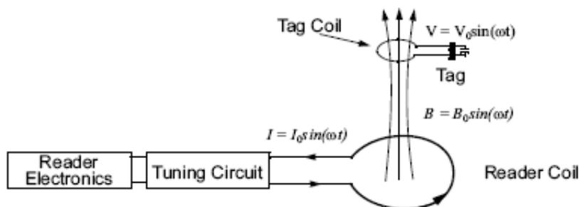
Figure 2: Inductive Antenna
