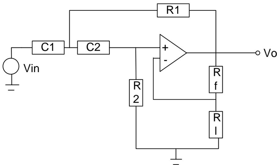
$$H(s) = \frac{V_0}{V_{in}} = \frac{A_0 S^2}{S^2 + \left[ \frac{1-A_0}{C_1 R_1} + \frac{1}{C_1 R_2} + \frac{1}{C_2 R_2} \right] S + \frac{1}{C_1 C_2 R_1 R_2}}$$
