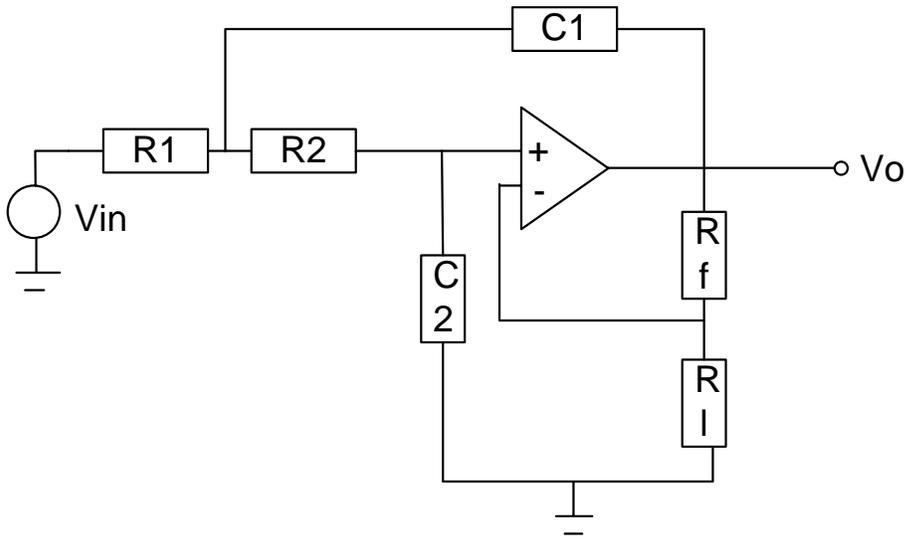
$$H(s) = \frac{V_0}{V_{in}} = \frac{A_0 / C_1 C_2 R_1 R_2}{S^2 + \left[ \frac{1 - A_0}{C_2 R_2} + \frac{1}{C_1 R_2} + \frac{1}{C_1 R_1} \right] S + \frac{1}{C_1 C_2 R_1 R_2}}$$
