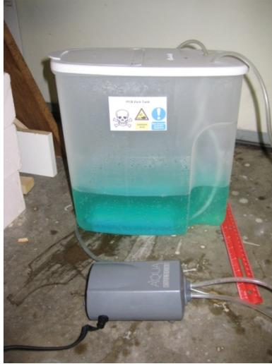
*Hydrochloric Acid Solution with Bubbler*
