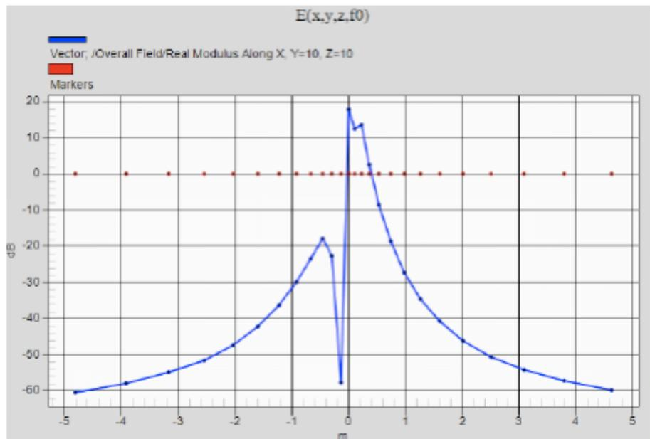
The tank is located at the 0 axis and extends 36 cm into the negative direction, and the edge source is located at the 0 axis, that is where the field is strongest. The graph indicates a large drop in decibels of the electric field within the water tank, hence the signal that penetrates through the water would be very weak.
